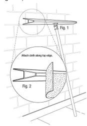
3. Start by applying the duster cloth to the black brush surface of the 3M™ Easy II Holder on one side and work your way across the 3M™ Easy II Holder. Make sure to align the edge of the duster with the edge of the black brush attachment surface (Figure 2).
